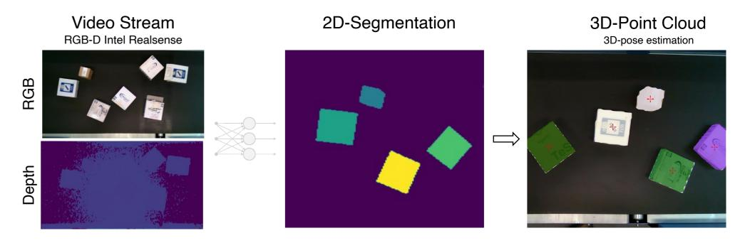
Overview of the image processing. First the parcels are segmented by a neuronal network. Then the 3D pose is estimated and sent to the robot.
