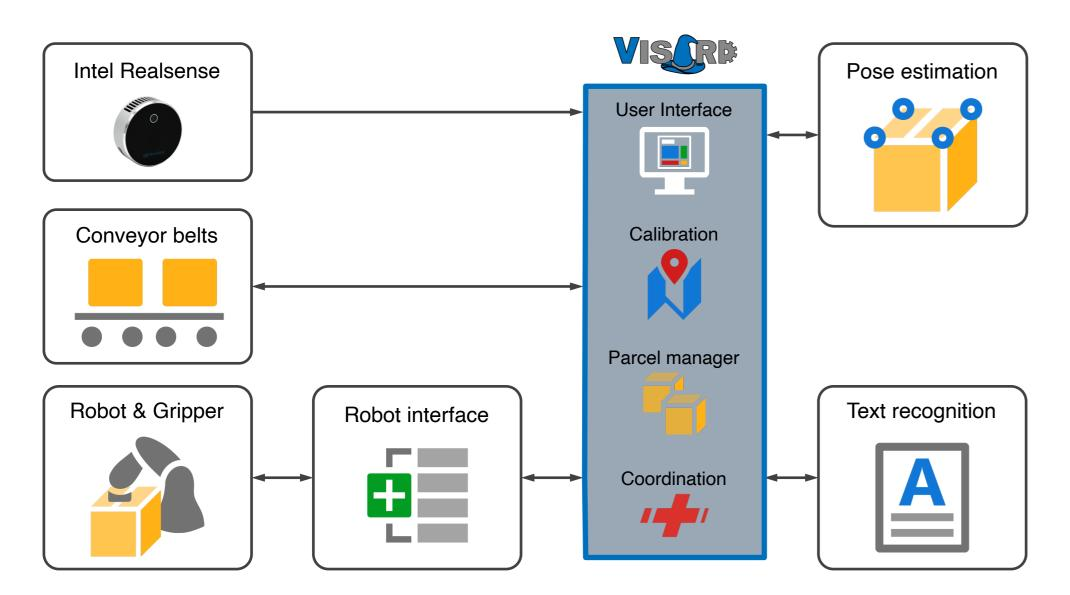
The system architecture is modular and allows many robot units based on the desired throughput. Modules communicate with gRPC/protobuf. CSEM's Visard builds the user interface and controls the whole process.
