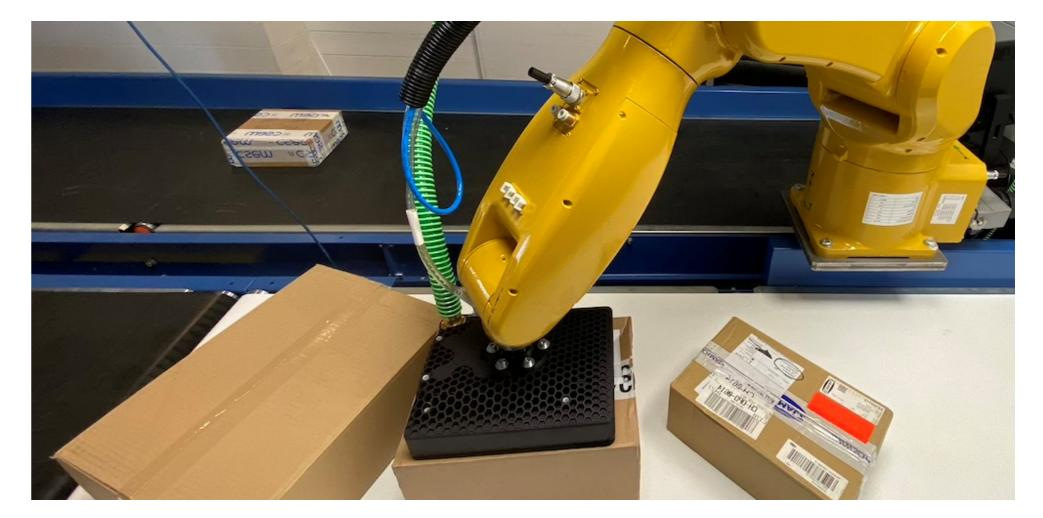
The 3D-printed vacuum gripper developed uses a combination of foam and suction cups with multiple gripping zones. Camera-robot calibration is achieved with an adapter plate with CCTags on the gripper.
